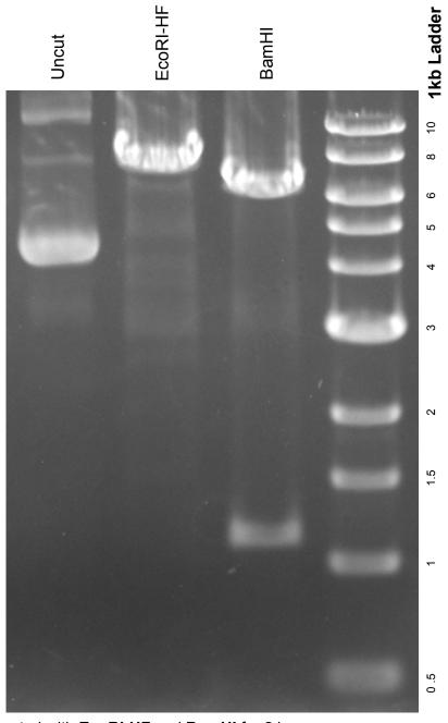
DNA digested with **EcoRI-HF** and **BamHI** for **2** hours Gel: 0.8% TAE stained with 100 ml 1X TAE and 5uL of ethidium bromide Ran for 1.5 hours at 80 volts
