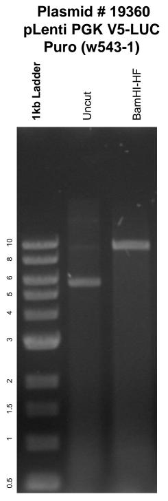
DNA digested with BamHI-HF single digest for **overnight** Gel: 0.8% TAE stained with 100 ml 1X TAE and 5uL of ethidium bromide Ran for 2 hours at **60** volts
