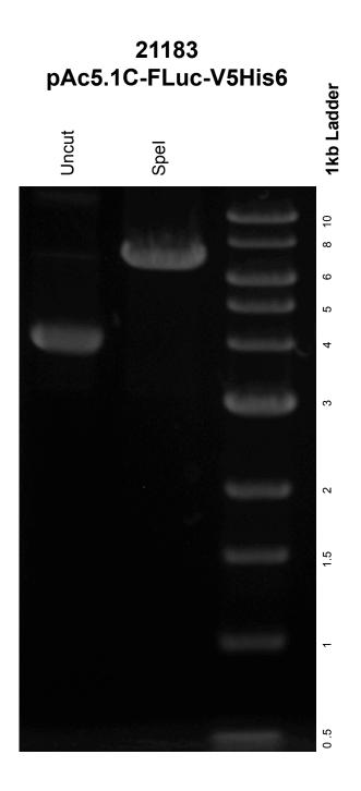
DNA digested with **Spel** for **1** hour Gel: 0.8% TAE stained with 100 ml 1X TAE and 5uL of ethidium bromide Ran for **1.5** hours at **80** volts
