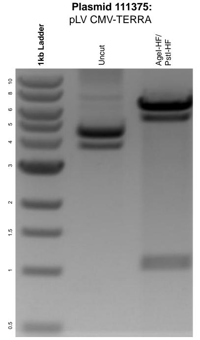
DNA digested with AgeI-HF/ PstI-HF double digest for **2 hours.** GeI: 0.8% agarose stained with 6 uL of ethidium bromide. Ran for 1.5 hours at 100 volts.
