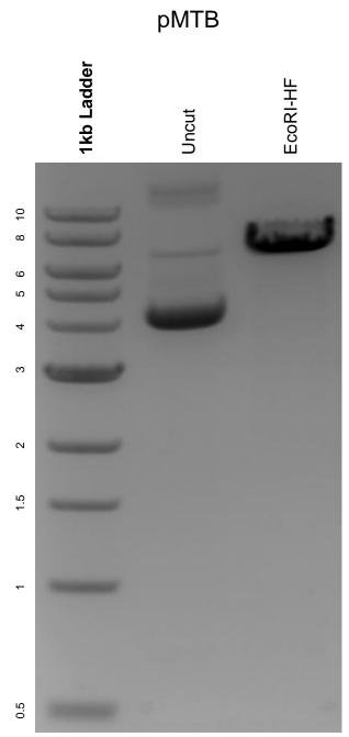
DNA digested with EcoRI-HF single digest for **2 hours**. Gel: 0.8% agarose stained with 6 uL of ethidium bromide. Ran for 1.5 hours at 100 volts.
