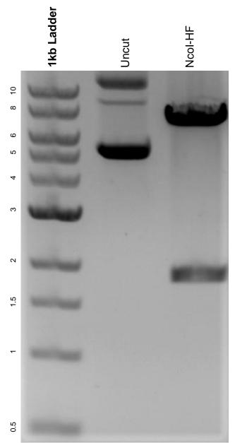
DNA digested with Ncol-HF single digest for **2 hours.** Gel: 0.8% agarose stained with 6 uL of ethidium bromide. Ran for 1.5 hours at 100 volts.
