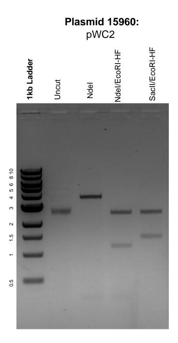
DNA digested with Ndel single digest and Ndel/EcoRI-HF and SacII/EcoRI-HF double digests for **2 hours**.
