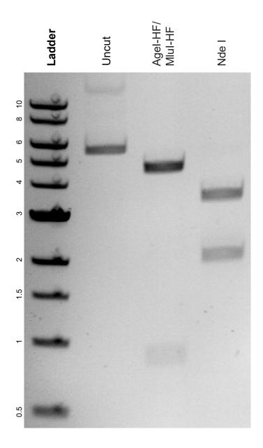
DNA digested with a Nde I single digest and a AgeI-HF/MluI-HF double digest for **1 hour**. GeI: 0.8% agarose stained with SYBR Safe. Ran for 1.25 hours at 100 volts.
