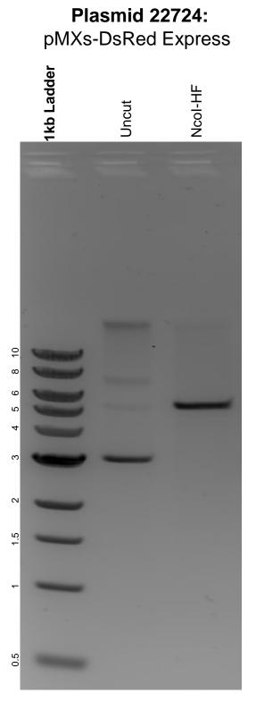
DNA digested with Ncol-HF single digest for **2 hours**. Gel: 0.8% agarose stained with 5 uL of ethidium bromide. Ran for 2 hours at 100 volts.
