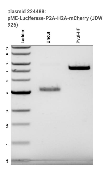
DNA was digested for 1 hour and run on a 0.8% agarose gel stained with SYBR Safe for 1 hour and 15 minutes (100 volts).
