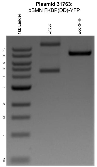
DNA digested with EcoRI-HF single digest for **2 hours.** Gel: 0.8% agarose stained with 6 uL of ethidium bromide. Ran for 1.5 hours at 100 volts.
