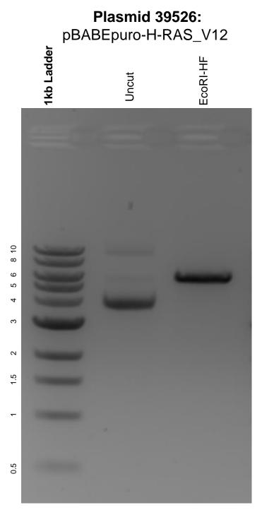
DNA digested with EcoRI-HF single digest for **2 hours.** Gel: 0.8% agarose stained with 5 uL of ethidium bromide. Ran for 1.5 hours at 100 volts.
