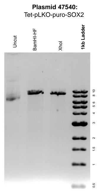
DNA digested with BamHI-HF and Xhol single digests for **2 hours.** Gel: 0.8% agarose stained with 5 uL of ethidium bromide. Ran for 2.5 hours at 60 volts.
