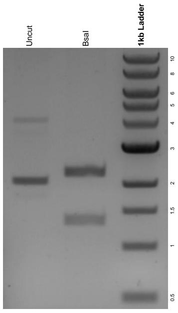
DNA digested with Bsal single digest for **2 hours**. Gel: 0.8% agarose stained with 6 uL of ethidium bromide. Ran for 1.5 hours at 100 volts.
