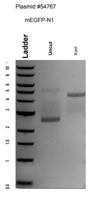
DNA digested with **Kasl** single digest for **1 hour**. Gel: **0.8%** agarose stained SYBR Safe. Ran for **1.15** hours at **100** volts.
