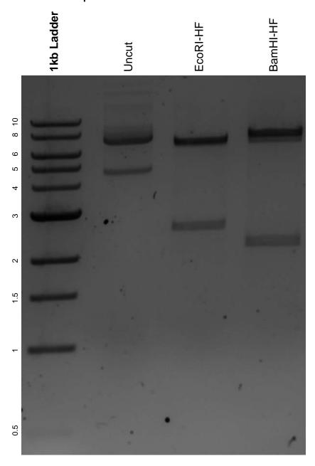
DNA digested with EcoRI-HF and BamHI-HF single digests for **2 hours**. Gel: 0.8% agarose stained with 5 uL of ethidium bromide. Ran for 1.5 hours at 100 volts.
