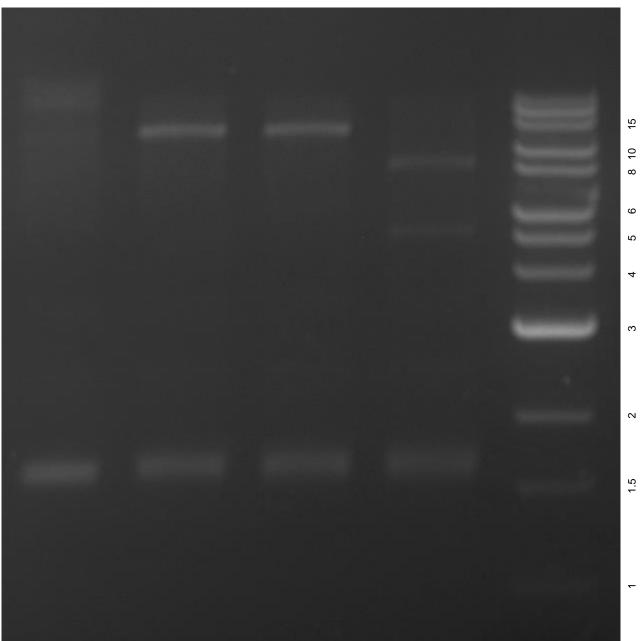
DNA digested with NotI-HF single digest, Xbal single digest, and NotI-HF / Xbal double digest for **1.5 hours.** Gel: 1% agarose stained with ethidium bromide. Run for 1.75 hours at 80 volts.
