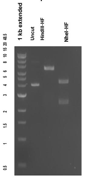
DNA digested with **HindIII-HF** and **NheI-HF** single digest for **1 hour**. Gel: **0.8%** agarose stained SYBR Safe.
